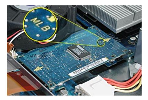
2. Reinstall the two ATA controller clips. (Figure 6)
